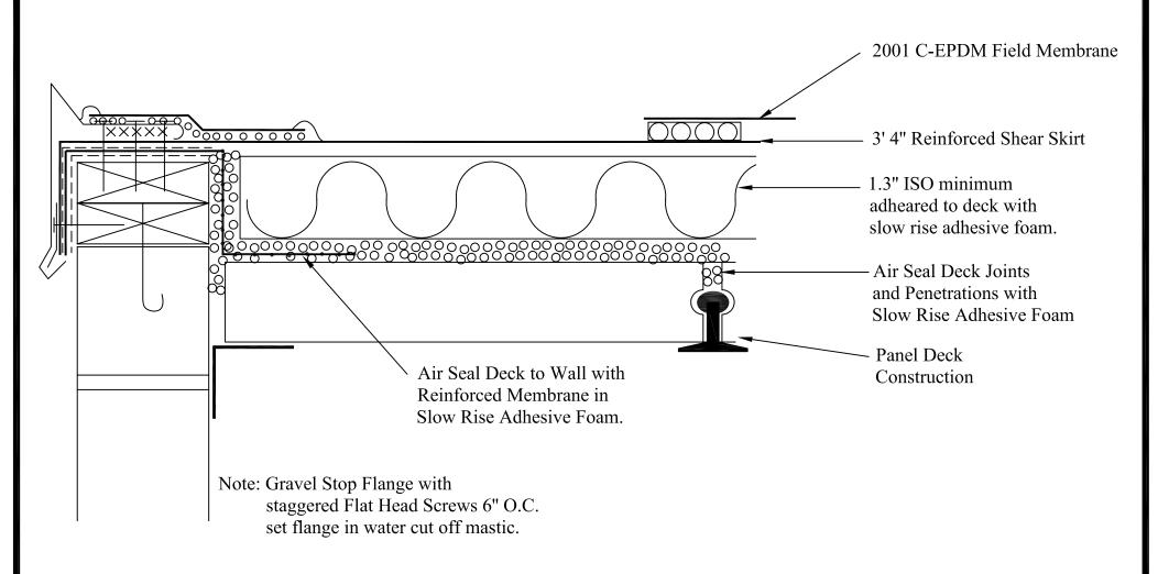
Option: Additional layers of insulation adhered with slow rise adhesive foam.
