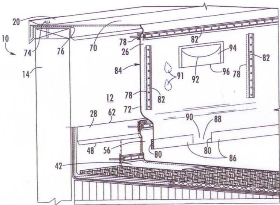
The bottom of the upper wall flashing has weep openings below the through-wall metal flashing to let condensation weep out and let air into the wall flashing for controlled air exchange drying.
