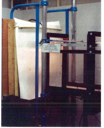
An air cannon above shoots a hail ball through a 10" speed recording chamber at a roof surface
